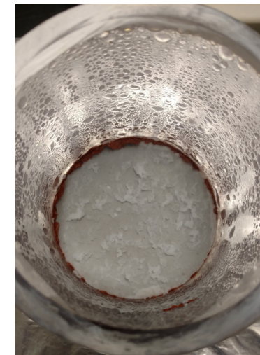
Etched aluminum with synthetic water before boiling
