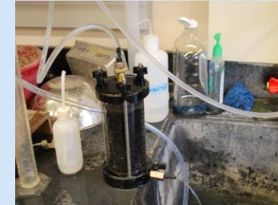
Figure 3. Assembly of Constant Head Hydraulic Conductivity Test
