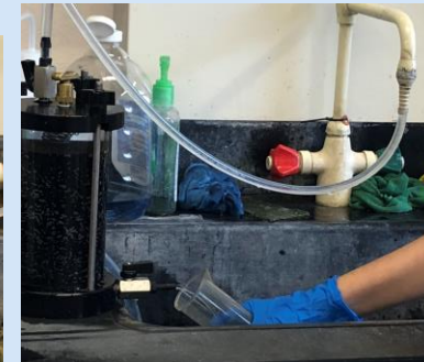
Figure 4. Collection of Water from Permeameter for Hydraulic Conductivity Measurements
