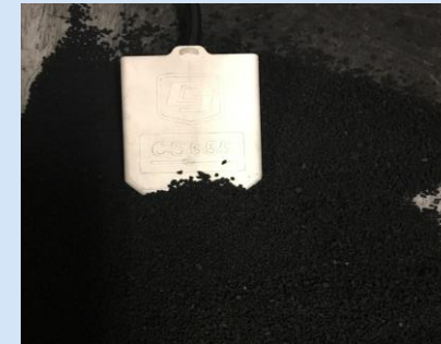
Figure 5. Volumetric Water Content Measurements of Granular Activated Carbon (GAC) Using Reflectometer
