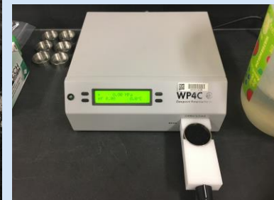
Figure 6. Matric Potential Measurements of Granular Activated Carbon (GAC)
