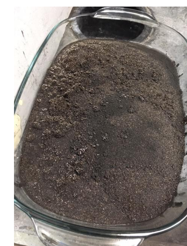
Figure 1.5 Final MnOx-coated sand
