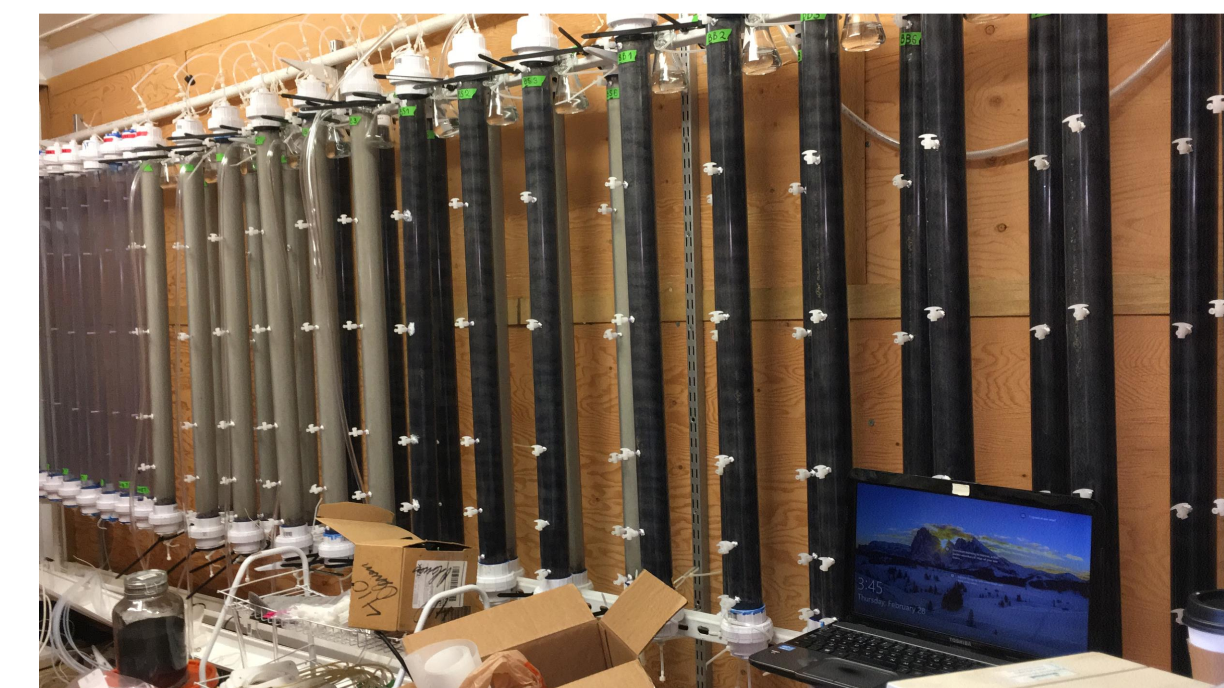
Figure 1.9 Field installation of upscaled MnOx
