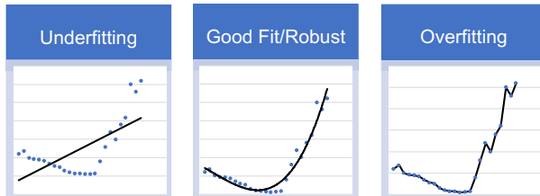
Figure 1. A visual representation of how a predictive model can be under- or over-fit if too little or too much data is used to train a NN model
