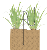
Fig. 3. Pushpoint sampler is inserted in a wetland.
