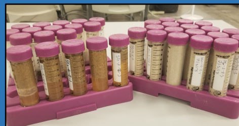
Figure 3. 1:5 saltgrass:distilled water solutions (left) and ground saltgrass (right).
